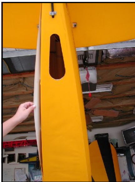
Air exit for canister use
